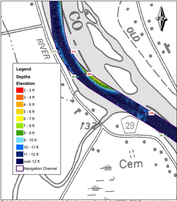
The bathymetry shown herein is based on a bathymetric survey performed by the NYSCC in 2012. The navigational design depth of the Champlain Canal is 12 feet.
