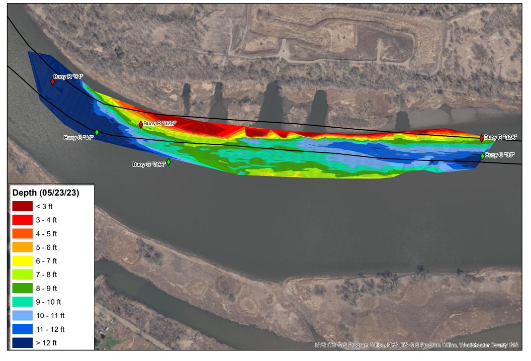
2023 Dredge Chart New York State Canal Corporation Eastern Division, Section 2, Waterford Pool at Lock E6 to E7 Depths are from the published pool elevation of 184 BCD Data Collected by: NYSCC Eastern Division Date of Survey: May 23, 2023 Actual Depth on date of survey: 185.2 BCD
