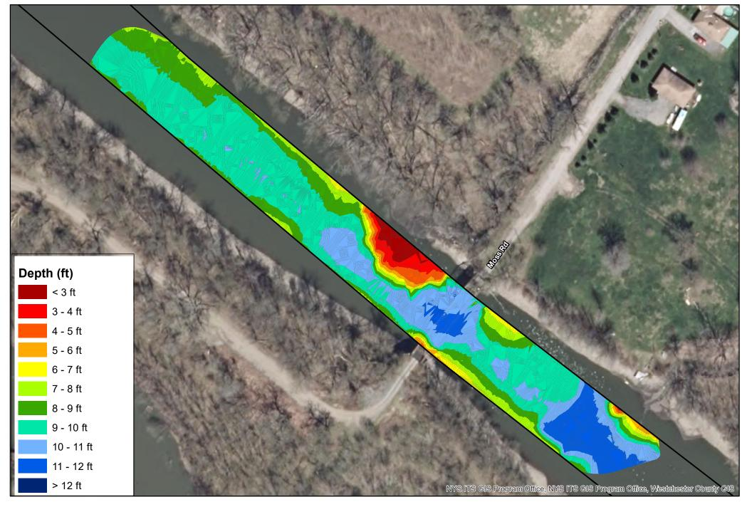
2023 Dredge Chart New York State Canal Corporation Eastern Division, Section 4 Utica Pool at Lock E18 to E19 Depths are from the published pool elevation of:383 BCD Data Collected by: NYSCC Eastern Division Date of Survey: May 18, 2023 Actual Depth on date of survey: 384.5 BCD
