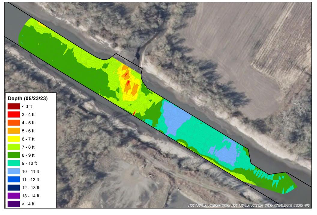
2023 Dredge Chart New York State Canal Corporation Eastern Division, Section 4 Utica Pool at Lock E19 to E20 Depths are from the published pool elevation of: 404 BCD Data Collected by: NYSCC Eastern Division Date of Survey: May 23, 2023 Actual Depth on date of survey: 403.8 BCD
