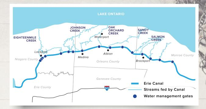
**But how does it work?** The Erie Canal in Western New York is an entirely man-made channel (unlike other regions where the Canal follows the course of a natural river). The Lake Ontario tributaries connected to the Canal serve as an outlet for the Canal's water management gates – which can be raised or lowered to manipulate water levels in the Canal for navigation, and are used to drain the Canal during the winter for maintenance.
